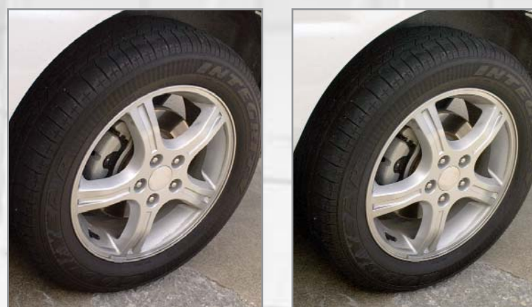
70% Inflated 100% Inflated It may be difficult to recognize an under-inflated tire
