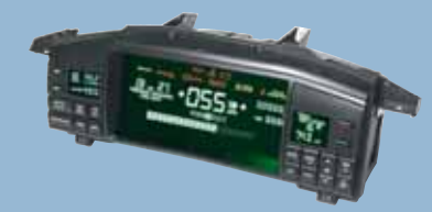
Electronic Dashboards can be both digital and analog. They function in a similar manner to mechanical dashboards but operate electronically.
