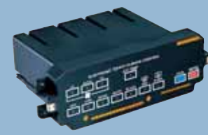
Climate Control Computers are designed to manage the heating ventilation and air conditioning of the vehicle. They are also used as an interface with the Body Computer.
