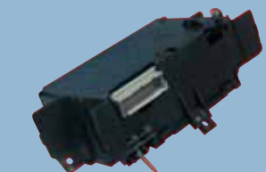
Ride Control Computers are programmed to modify the suspension characteristics of the vehicle to compensate for road and driving conditions.
