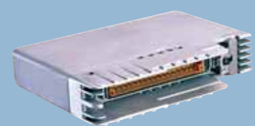
ABS Computers are programmed to compensate for tire lock up by modulating the braking action.
