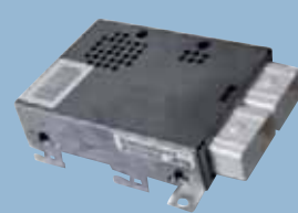
Body Control Computers are programmed to manage and control several devices such as theft deterrent, lighting, climate control, intermittent wipers and vehicle mileage.
