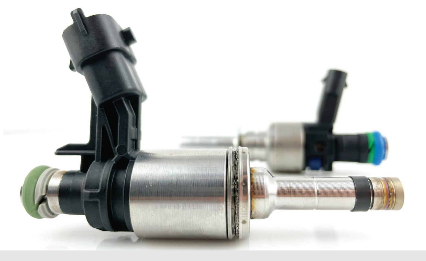
Most GDI injectors can't be remanufactured because they can't be disassembled to replace worn and failed components
