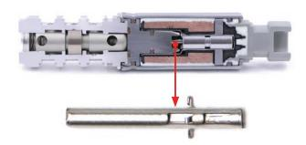
Uses an aluminum internal shaft which can deform over time and alter the timing of the valves
