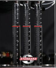
Standard® Injectors are tested and calibrated for consistency to optimize performance
