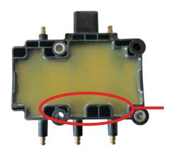
No cracks after temperature test
