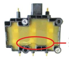
OE epoxy cracks after temperature test
