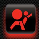
Airbag Fault: If this light stays illuminated after starting it indicates that the vehicle has found a fault in the airbag system and the computer has set a code. Professional repair of the supplemental restraint system is recommended.
