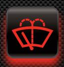
**Washer Fluid Reminder:** Indicates washer fluid is low. Fill washer fluid reservoir. The cap has a symbol that looks like a windshield. Some vehicles have separate reservoirs for front and rear window washers.
