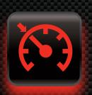
**Cruise Control:** Indicates that the cruise control system is engaged while the vehicle is driving.
