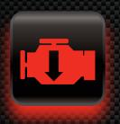
**Reduced Power Warning: Indicates Engine Computer has** limited engine power output. The **ECM** has many levels of reduced power depending on what component has failed in its control system. Usually requires diagnosis with a professional scan tool.
