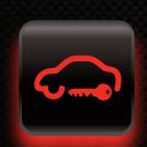
**Security Alert:** If the symbol lights momentarily it may mean the ignition switch is locked and will need the proper transponder-equipped key to re-start. If the symbol is visible when the vehicle is on, it typically means a malfunction in the security system.
