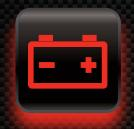
**Battery/Charging Alert:** Indicates voltage level is below normal level and the vehicle's charging system is not functioning properly. Check battery terminals, alternator belt, and battery condition.
