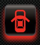
**Door Ajar:** Indicates a door (including hood and trunk) is not closed. Open and close all doors, including hood and trunk. If vehicle is left in this condition overnight, it can drain the battery.
