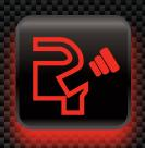
**Gas Cap:** The check gas cap light indicates that the gas cap is not tightened properly. If not addressed, quite often the Check **Engine Light will also illuminate.**
