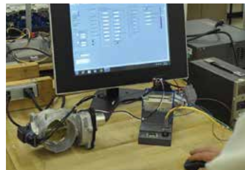
TechSmart® engineer performing TPS output test
