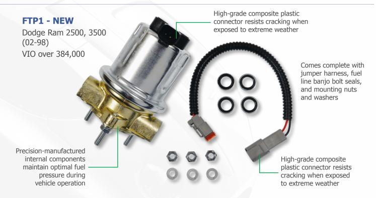
**Tech Tip:** Fuel transfer pump pressure should be 8-10 PSI during cranking and more than 5 PSI during vehicle operation.
