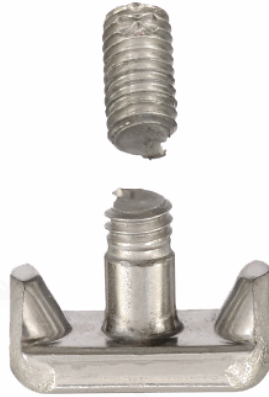
Broken OE Bolt
