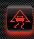
**Traction Control or ESP:** Illuminates when the vehicle's traction control/antiskid or electronic stability system is in use. Usually an indicator that conditions are slippery.
