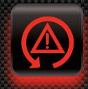
**ESP Fault:** Indicates that there is a problem with the vehicle's traction control/anti-skid or electronic stability system.
