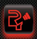
**Gas Cap:** The check gas cap light indicates that the gas cap is not tightened properly. If not addressed, quite often the Check **Engine Light will also illuminate.**
