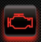
**Check Engine or Malfunction Indicator Light (MIL):** Indicates the engine computer has set a Diagnostic Trouble Code (DTC). Usually requires diagnosis with a professional scan tool.
