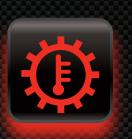
**Transmission Temperature:** Transmission is operating at higher than optimum temperature as transmission fluid is hotter than normal. Check transmission fluid level and engine coolant level.
